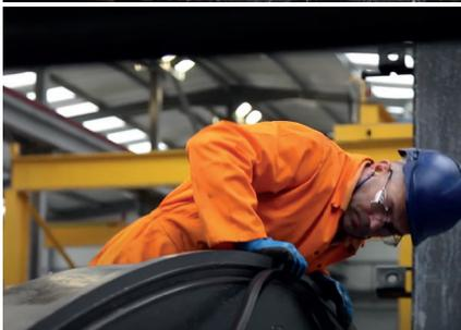
After the corners continue with the long sides (circumferential joint sides) beginning from the middle. Take care that you equably distribute the gasket material along the groove and check that all sections are properly clipped in.
