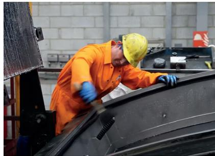
Then continue with the remaining small sides (longitudinal joint sides), also starting from the middle and going towards the corners. Again take care that you equably distribute the material along the groove and check again that all sections are sufficiently clipped in.
