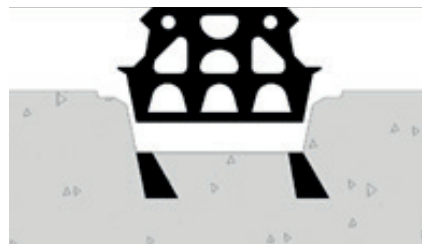
Repair profile to be inserted and glued into the groove
