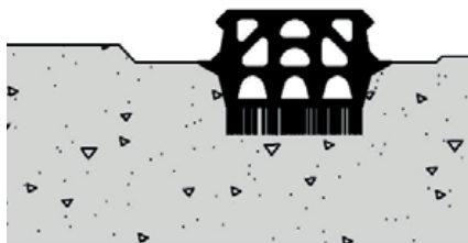
Installation situation of fiber anchored profile
