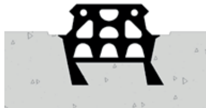
Installation situation of anchored profile
