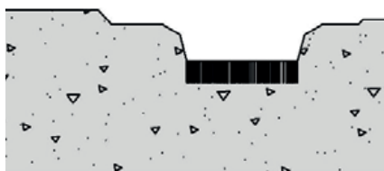
Groove cross-section after removal of damaged gasket frame
