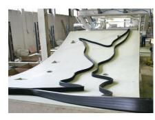
Prior to installation of the gasket into the groove it should be positioned somewhere on top of the segment and nearby the groove so that it can be quickly and easily pushed into the groove once the wet bed of glue has been applied.
